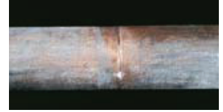
TUBE SUPPORT WEAR Caused by the tube/support contact. Although this phenomenon is quite rare, it must be quickly detected.
