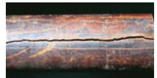
STRESS CRACKING Longitudinal or intergranular cracks caused by high water flow.
