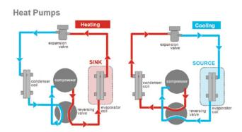
Heat pumps use electricity to move energy around to cool or heat the space. In cooling mode, they move heat inside your building to outside. In heating mode, a reversing valve changes the flow of energy and moves outside energy (even if its cold outside) to inside the building.
