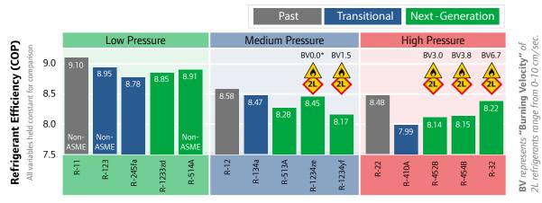
\*R-1234ze is not flammable at room temperature, so its BV is zero by definition. It does, however, become flammable at temperatures above 30°C (86°F).
