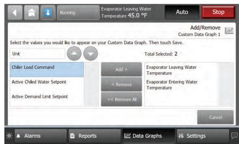
Figure 26. Add/Remove screen example
