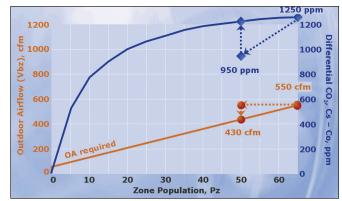
Figure 1 (left): Standard 62-2001: required OA flow and CO<sub>2</sub> level. Figure 2 (right): Standard 62.1-2004: required OA flow and CO<sub>2</sub> level.
