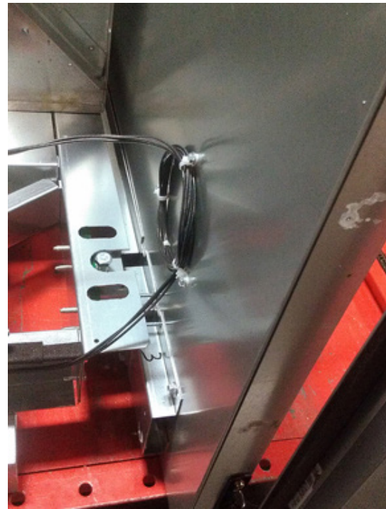
Figure 19. Remove screw ties holding high voltage wiring harness
