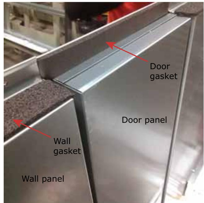
Figure 10. Gasket details at top corner
