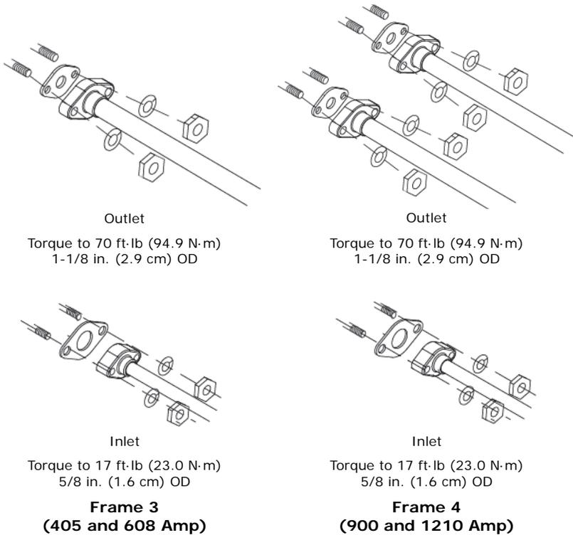
Refrigerant coolant lines connect to the cabinet through flange fittings located on the rear of the cabinet. A panel must be removed to provide access to the flange connections. If you have removed the refrigerant cooling lines for field disassembly or repairs use the following steps to re-connect the coolant lines to the cabinet (see [Figure 14](#)).
