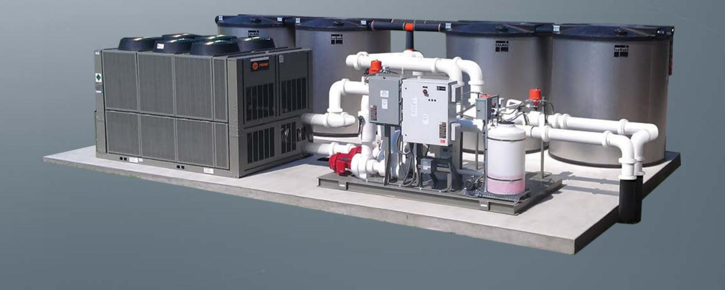
The Trane Thermal Battery system is a Trane controlled chiller plant enhanced with **thermal energy storage**. The chiller plant operates like a battery, charging Ice Bank® energy storage tanks when excess or inexpensive energy is available. And discharging when demand is high or price is high or when the utility asks for the discharge to occur.
