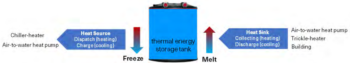
Figure 4. Thermal energy storage tank operation
