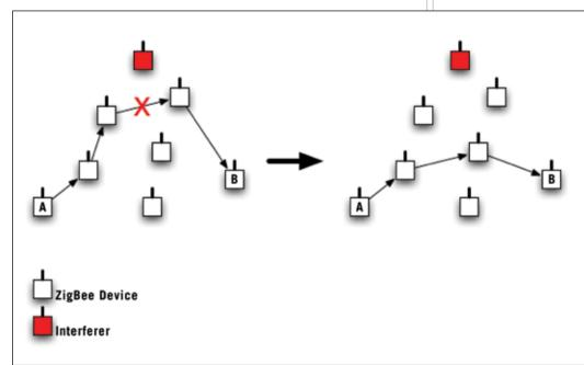
the network manager. This device may direct the network to leave the channel it is currently using and form on another channel.
