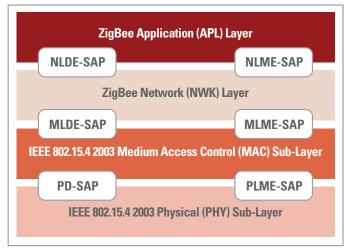
Figure 1 - The ZigBee Stack
