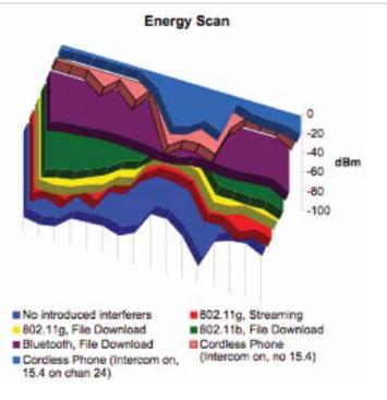
Figure 10 - Interference Sources
