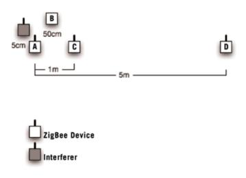
Figure 9 - Test Setup
