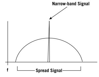
Figure 3 - Spread-Spectrum Signal
