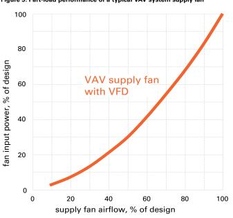
Figure 5. Part-load performance of a typical VAV system supply fan
