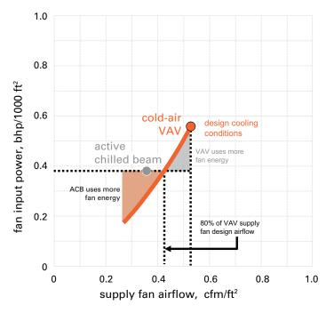
Note: For the cold air VAV system (48°F primary air, rather than conventional 55°F), assumes the ductwork has been downsized for first cost savings—so total static pressure remains the same at 4 in.  $H_2O$ —and assumes 60% fan efficiency.
