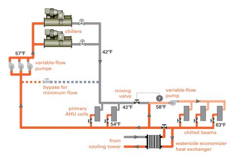
Note: Other plant configurations have been used—such as putting the primary AHU coils and chilled beams in series or putting chillers in series and diverting some of the warmer water leaving the upstream chiller to serve the chilled beams—and they can provide energy benefits over this example configuration, but they also increase complexity.
