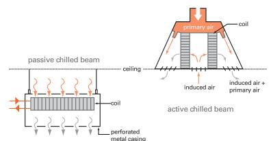
Figure 2. Examples of active chilled beams
