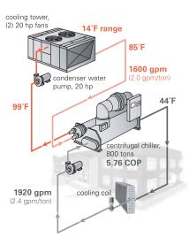
cooling tower and condenser water pump exceeded the chiller's additional power consumption. Ultimately, the projected energy consumption for the entire chilled water system is 8 percent less than the base design:
