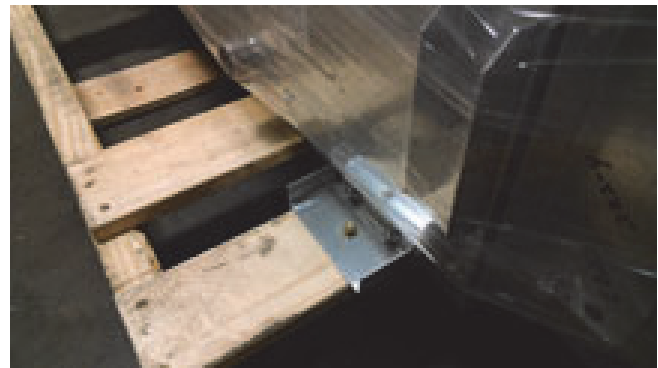
Figure 11. Do not use skid tie down for lifting
