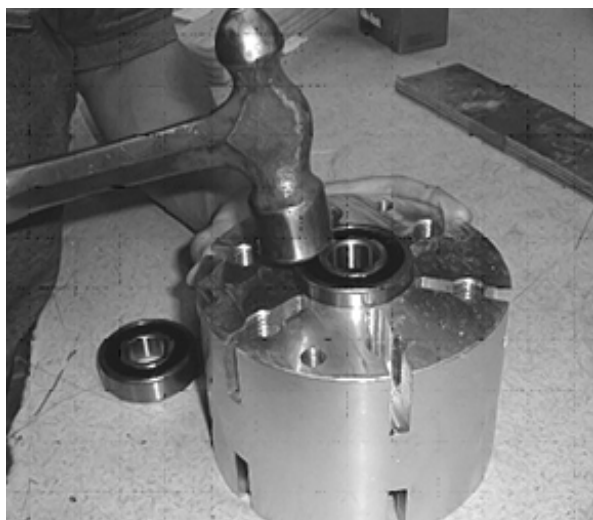
Figure 180. Tap outer race of new bearing, alternating sides
