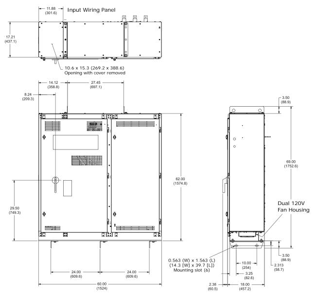
Figure 10. Drive cabinet dimensions: Frame 4, in. (mm)
