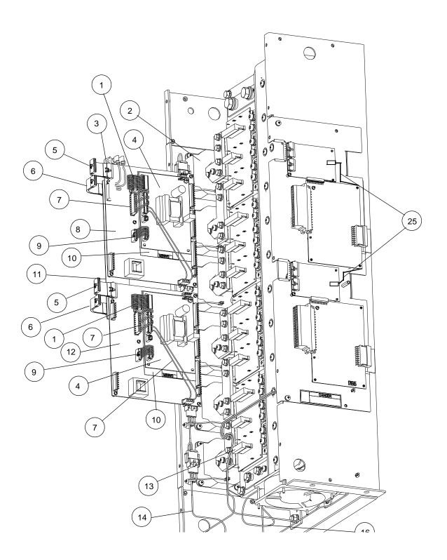
Figure 4. Power module component locations door closed: Frame 3 units
