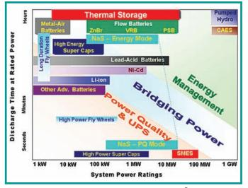
Figure 1: Different types of energy storage systems.<sup>7</sup>
