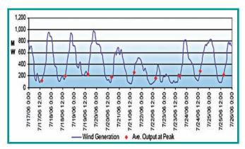
Figure 6: Design week wind generation output.
