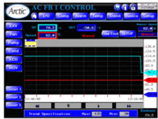
Figure 18. Fan control screen
